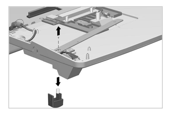
Figure 7-38. Removing the Docking Lever
